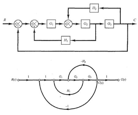
In this system there is only one forward path between the input R(s) and the output C(s). The forward path gain is
