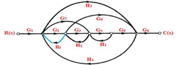
Obtain the closed-loop transfer function using Mason's gain formula.
