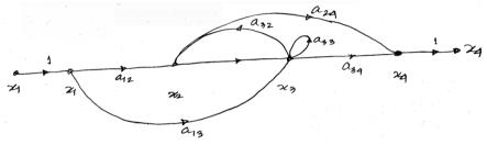
SFG of a multi input system can be constructed from the describing equations:
