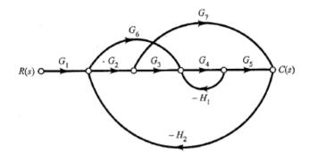
In this system, there are three forward paths between the input R(s) and the output C(s). The forward path gains are
