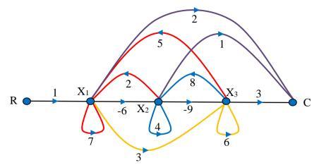
On the other hand, the signal flow graph can be given and the student is asked to obtain the system equations.
