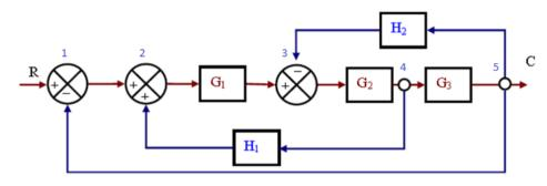
Choose the nodes to represent the variables say 1, 2, .. 5 as shown in the block diagram above. Connect the nodes with appropriate gain along the branch. The signal flow graph is shown below.
